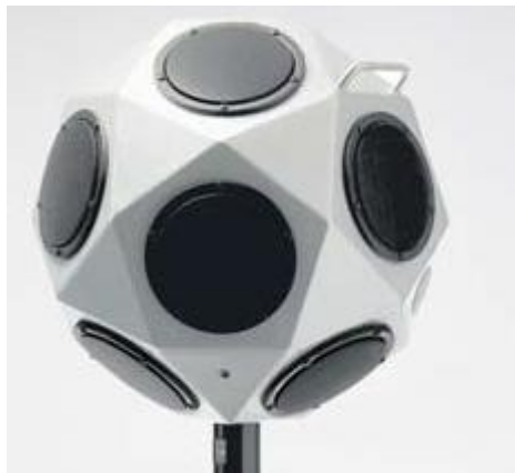
Fig. 3.37. Twelve-speaker omnidirectional sound source: a laboratory construction of pulsating sphere. Bruel & Kjaer Omni Power Sound Source - type 4292.
